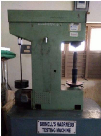
Fig. 3. Brinell's hardness testing machine.
